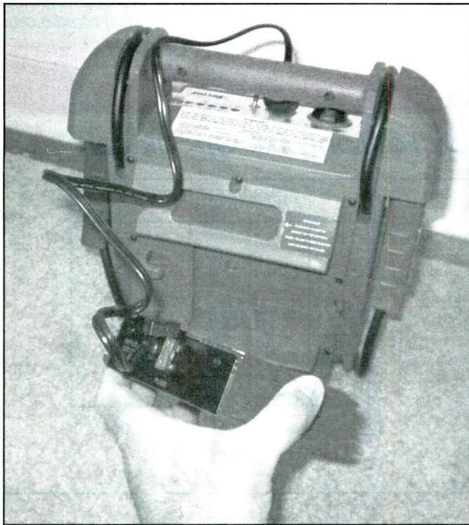
The 200-watt removable inverter has an easily accessible fuse on the back.
