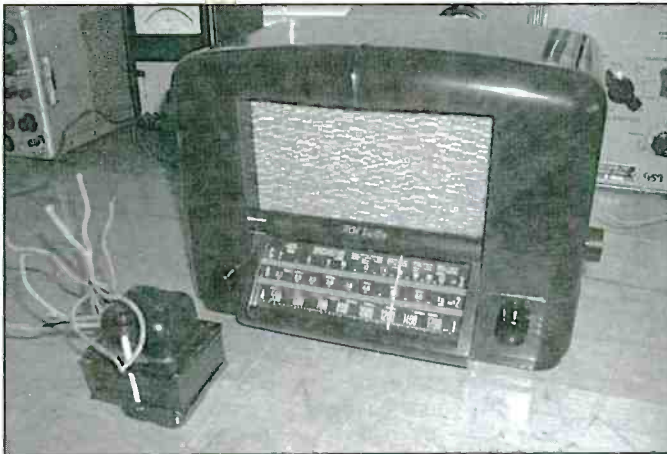
Photo 2. The RCA Model 5Q55 radio. The transformer is the defective original RCA transformer. Note the odd color codes used on the transformer leads.
