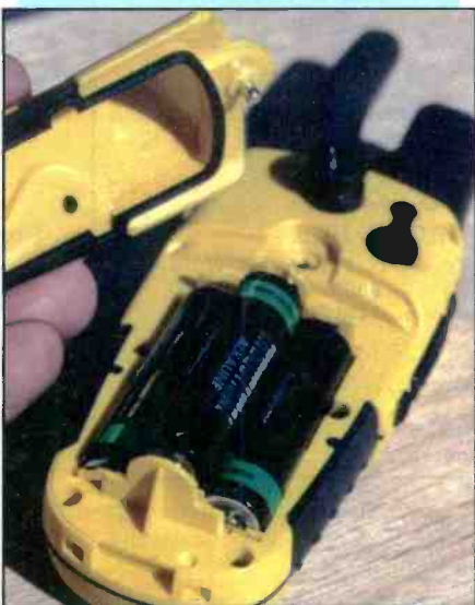
The battery compartment is double sealed against water intrusion.
