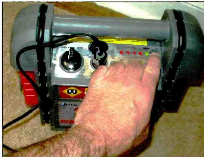
The top-mounted LED status lights.
